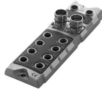
The expander module is designed for connecting up to 8 read/write heads: BIS L-3\_ \_ or BIS M-3\_ \_ can be selected using the rotary switch, depending on the processor (L or M). The read/write heads are selected electronically and are therefore not subject to wear. The process for selecting the read head can be monitored via feedback signals. 2 x 4 control signals help to select the desired read/write head.
